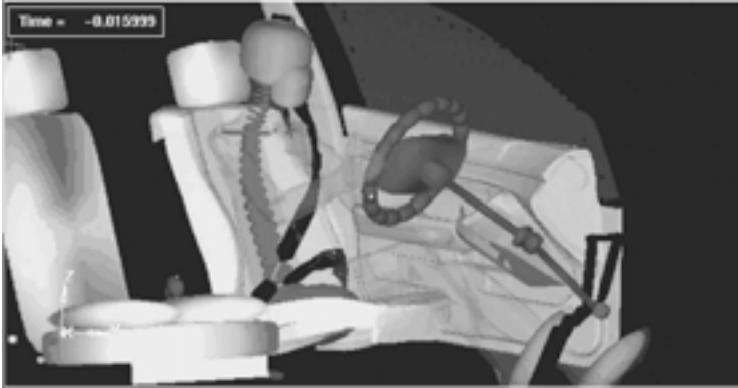
*Fig. 8: Accident reconstruction, initial position shown with transparent skin*
