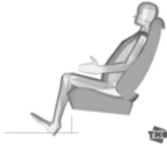
*Fig. 7b: Human body in rear impact at t=61 ms*
