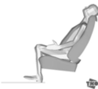
*Fig. 7c: Human body in rear impact at t=101 ms*
