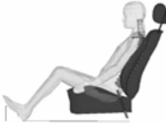
*Fig. 10: Vibration simulation with human model in standard car seat*
