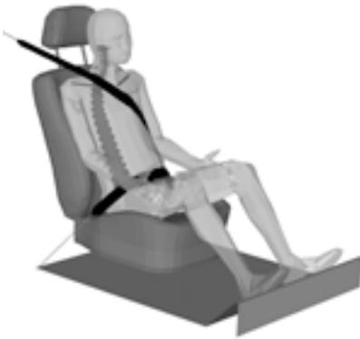
*Fig. 5: Human model restrained by finite element belts*
