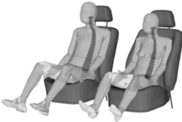
*Fig. 1: Human models representing a mid size male (left) and a small female (right).*
