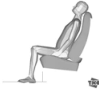
*Fig. 7d: Human body in rear impact at t=171 ms*
