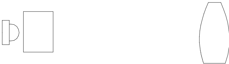
Figure 5: Vertical section through a proposed LED fog lamp. This module employs a LED, a lens, which directs the light into a certain area and a cylinder lens, which projects the light on the street.
