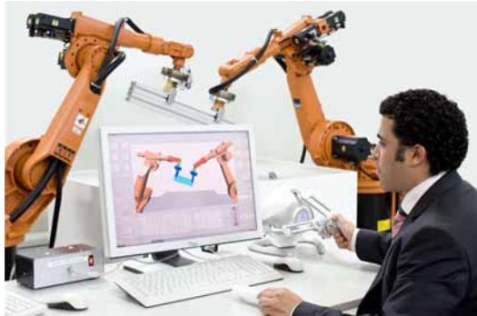
Figure 1.11: Universal workpiece based approach for programming of cooperating industrial robots (REINHART & ZAIDAN 2009)
