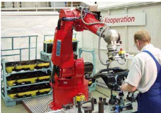
Figure 1.7: PowerMate assembly work-cell (SCHRAFT ET AL. 2005)
